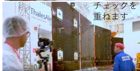
SENTINEL 1C Solar panel deployment
